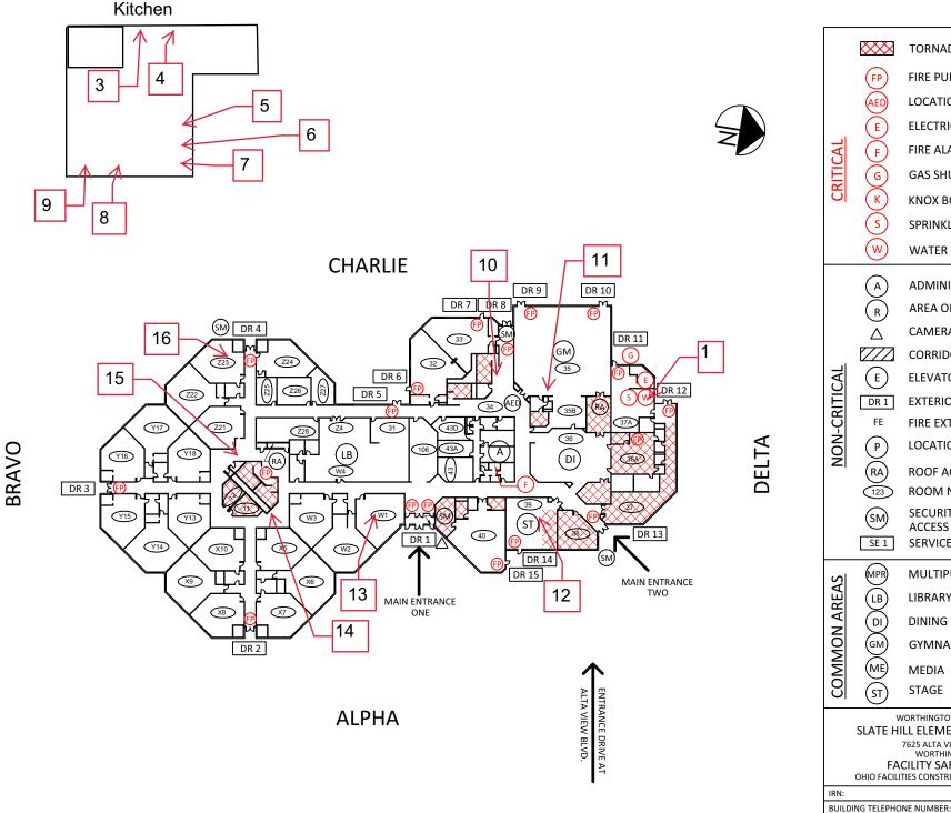
TORNADO EVAC. SITE FIRE PULL STATIONS LOCATION OF EXISTING AED **ELECTRICAL SHUTOFF** F FIRE ALARM PANEL G **GAS SHUTOFF**  $(\kappa)$ **KNOX BOX** SPRINKLER SHUTOFF WATER SHUTOFF ( A) **ADMINISTRATIVE SUITE** AREA OF REFUGE Δ **CAMERA** CORRIDOR (E) **ELEVATOR** DR 1 EXTERIOR DOORS FIRE EXTINGUISHER LOCATION OF BLUEPRINTS (RA) (123) **ROOF ACCESS POINT**
